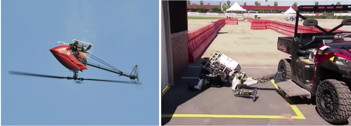
Figure 1.2: Left: an autonomous helicopter successfully performs inverted flight. Right: a humanoid robot fails to maintain balance while stepping out of a vehicle.
